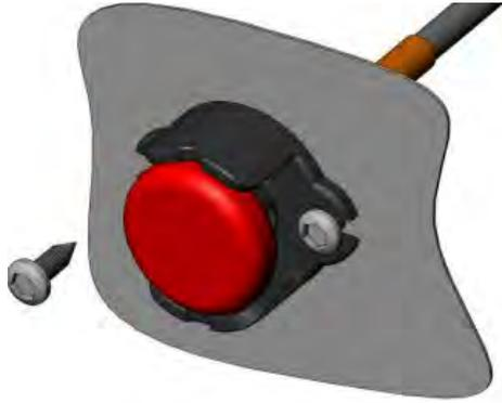
**Step 7:** With the padlock closed and the knob aligned, apply the safety seal if required for uses.
