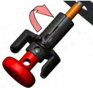
**Step 5:** Insert the support into the door sheet metal and close the padlock by rotating the harpoon (the red knob will return). Carry out some functional tests before fixing the plastic support. If necessary, screw or unscrew the support to adjust the stroke.
