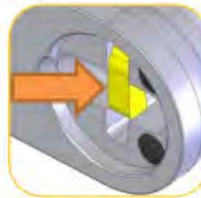
**Step 6:** Fix the support to the door sheet or to the panel using the screws provided. Check that the passing hole of the knob and that of the support are aligned in order to guarantee the passage of the safety seal.
