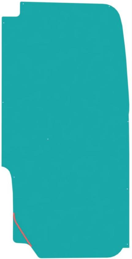
Cut along the profile shown above (located on the back of the panel) to use in 2019 and newer model year vehicles.
