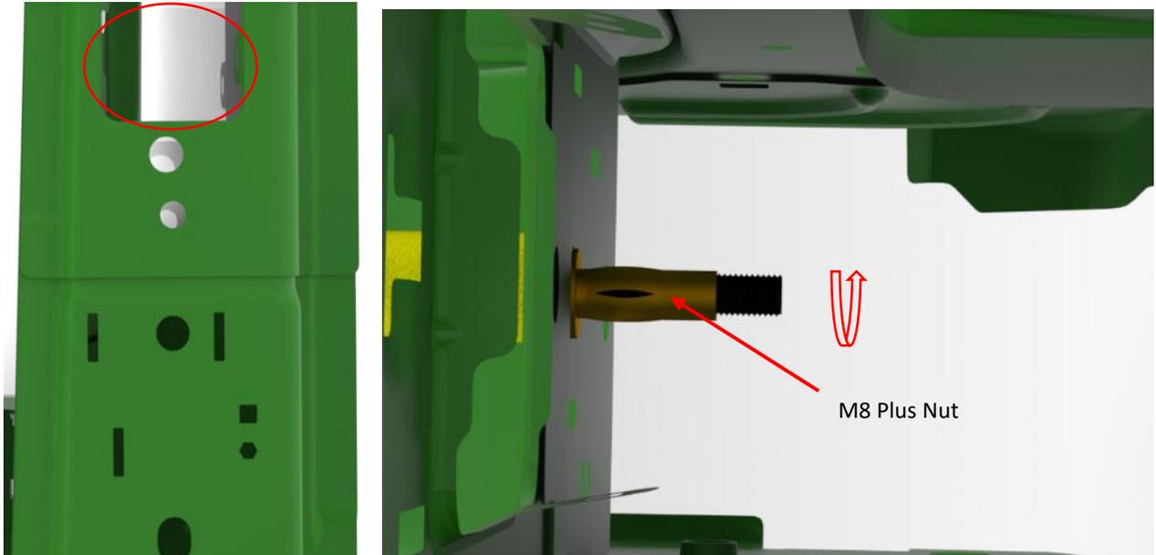
6. The hardware installed at the upper and lower fastening points in steps # 2 and #4, can now be tightly fastened.
