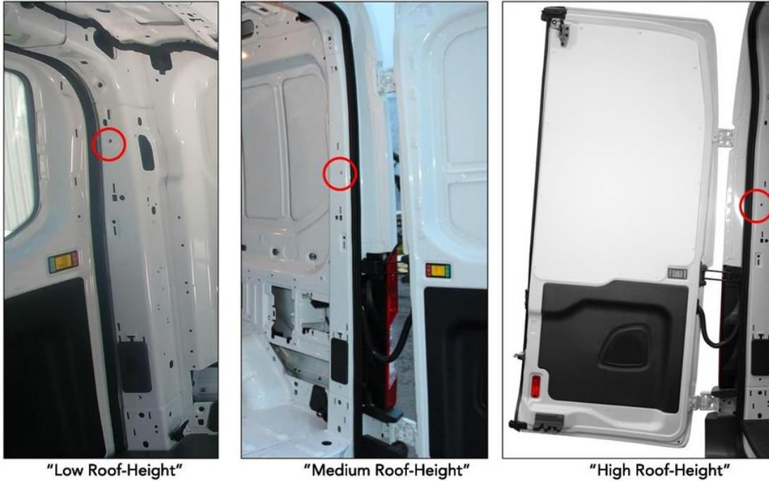
2. Fasten the handle in van using the hardware provided, in the order as shown below.
